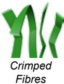
Polytan's LigaGrass system also has special crimped monofilament fibres which have been designed to trap the infill in place and reduce the amount of infill migration and infill displacement that tends to occur with artificial turf fields.
